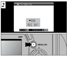
Check the size at which the image will be saved and then press the "MENU/OK" button. The trimmed image is saved as a separate file.
